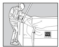
Attach the lifting straps to the transformer manufacturer's lifting lugs.
