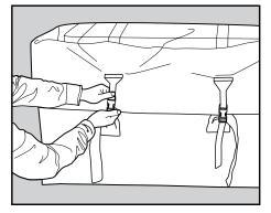
Fasten the cap buckles to the integrated buckles on the lower Transformer Containment Bag™.
