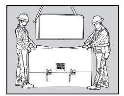
Hold the Transformer Containment Lay the (4) nylon webbing straps Bag™ open and lower the transformer into the bag. Detach the lifting straps from the manufacturer's lifting lugs.
