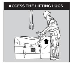
Release buckles on the short sides and pull up the cap on both ends to access the lifting lugs.
