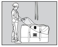
Place the cap over the Transformer Containment Bag™ for complete weather protection.
