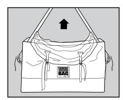
Lift the transformer by the lugs using the lifting straps with the Transformer Containment Bag™ attached as shown.
